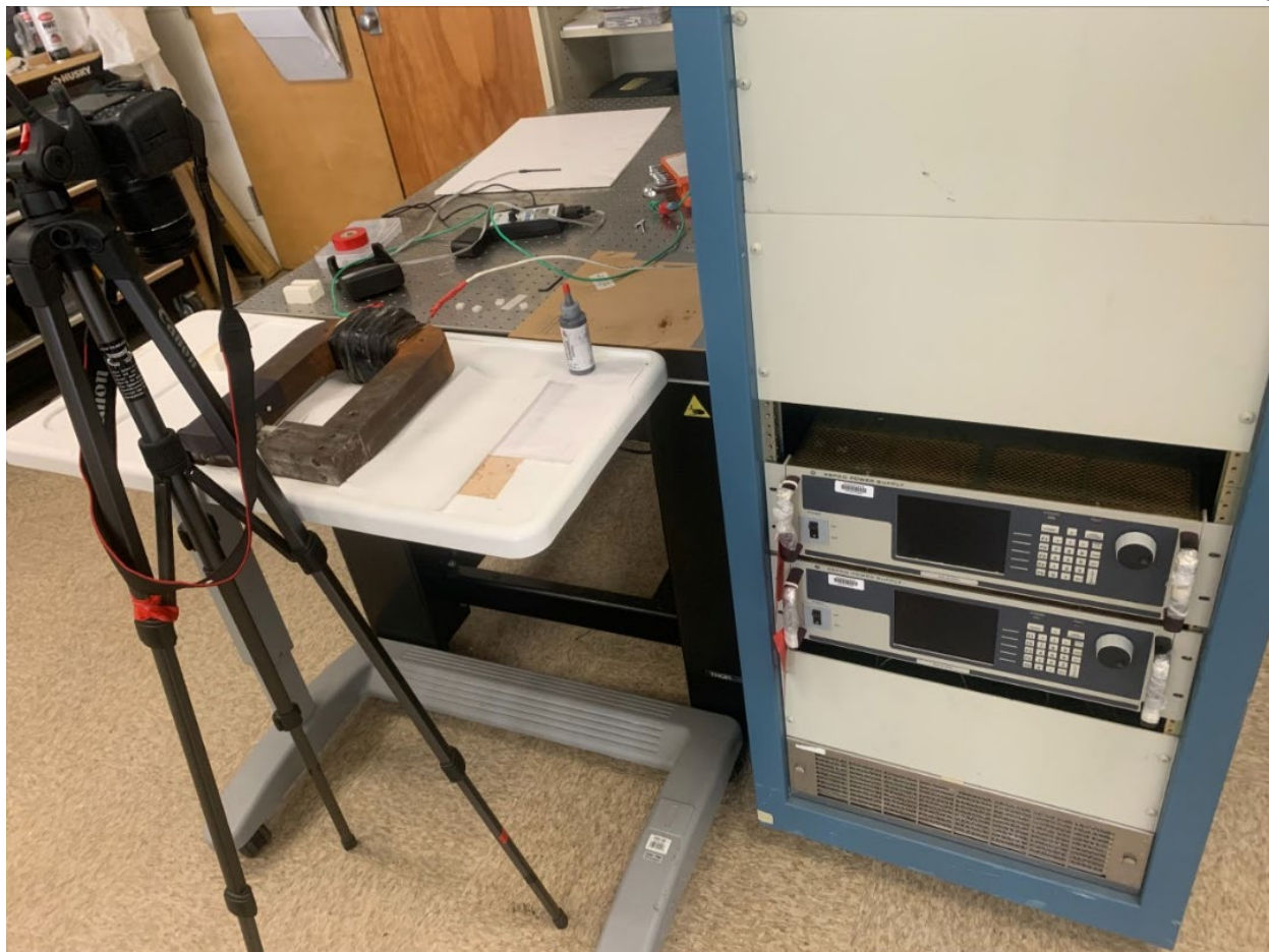
Figure 5. The experimental setup used to test the physical model. A pair of KEPCO power supplies wired in series, on the right, power custom electromagnet, on the left. The array of magnets is placed within the gap in the electromagnet. A camera records the magnet motion.
