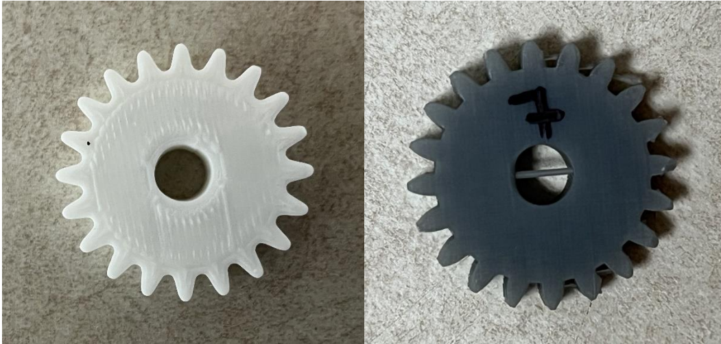
Figure 7: FDM Gear 7 Surface Quality
