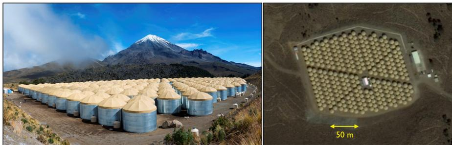
Figure 1.7: Side view [10] (left) and top view [11] (right) of the High-Altitude Water Cherenkov Gamma-Ray Observatory.
