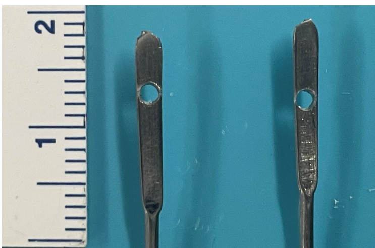
Figure 3.2: Current Cavity Electrode Design (Fe wires)
