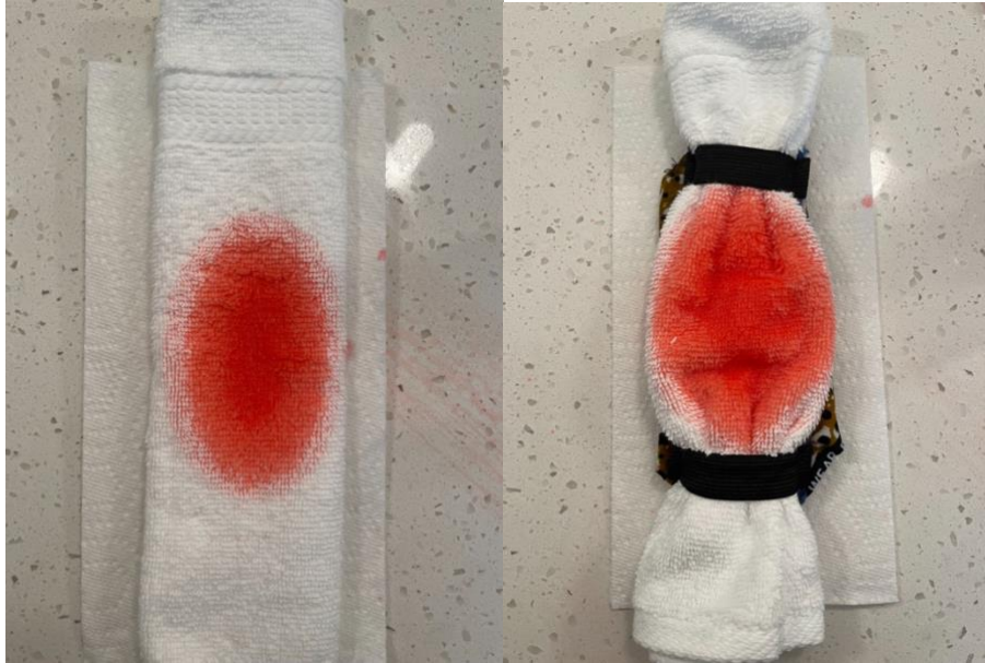
Figure 10. Comparison of Cloth by Itself with Cloth + WISSP Pad to Demonstrate Scrunching Phenomenon
