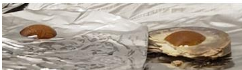
Figure 4.6 Polyimide Wetting on ZnO and Aluminum Foil Surface
