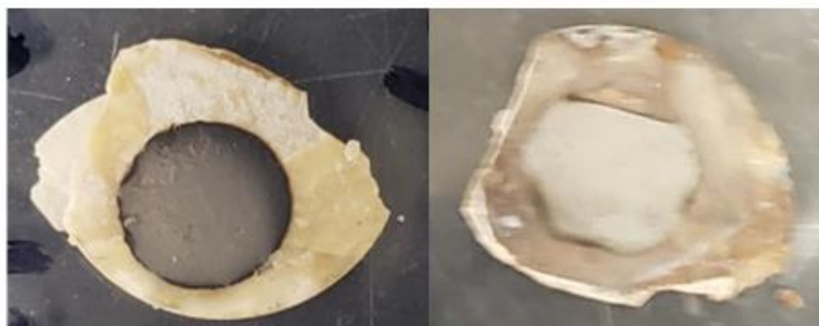
Figure 5.3 1-Step Polysol Composite Pellet Before and After Crosslinking
