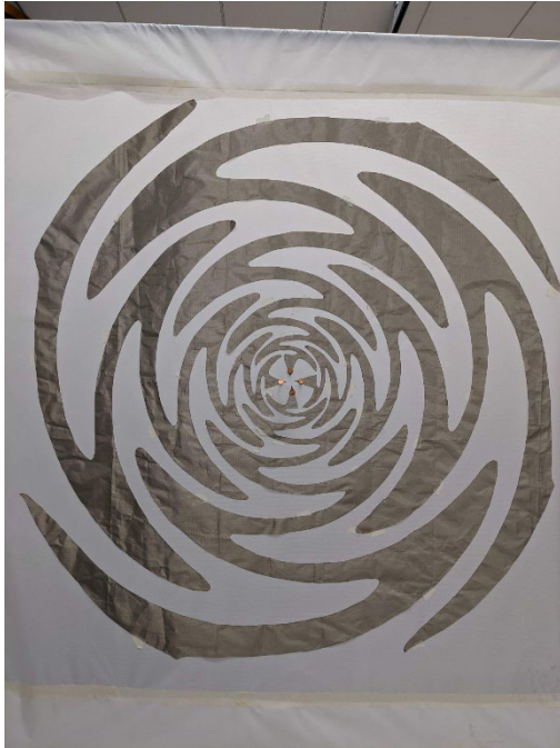
Figure 7: Half-scale model of a LF Sinuous antenna
