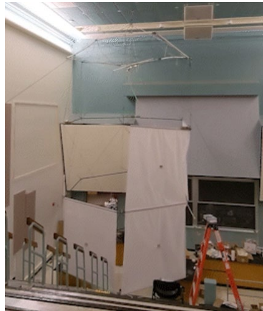
Figure 8: Half-scale model of deployable LF frame
