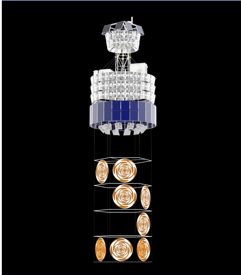
Figure 4: Rendering of PUEO's payload containing the MI and LF Instrument. [1]
