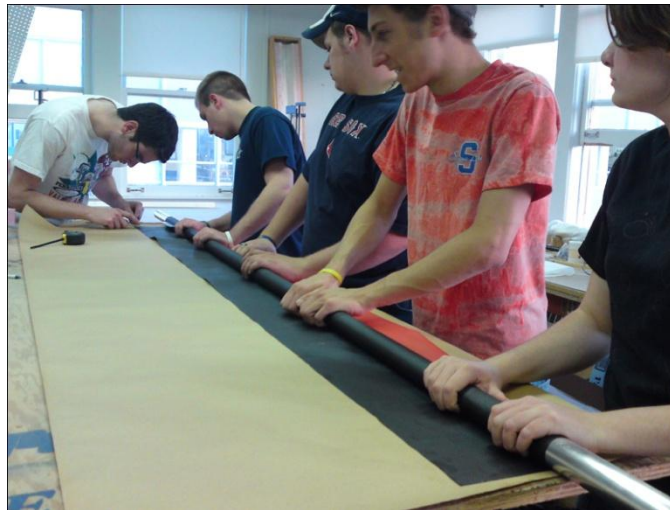
Figure 21: Students manufacturing carbon fiber tube
