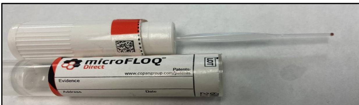
Figure 2. Copan microFLOQ ® Direct Swab tip showing a minute amount of blood on the tip.
