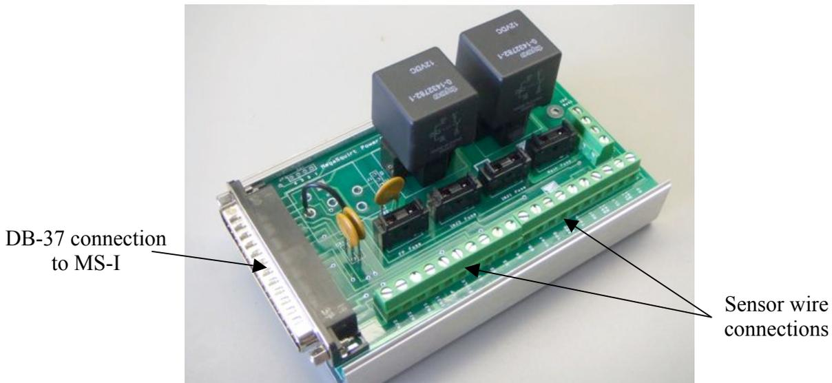
Figure 4.3 The stimulator board assembled
