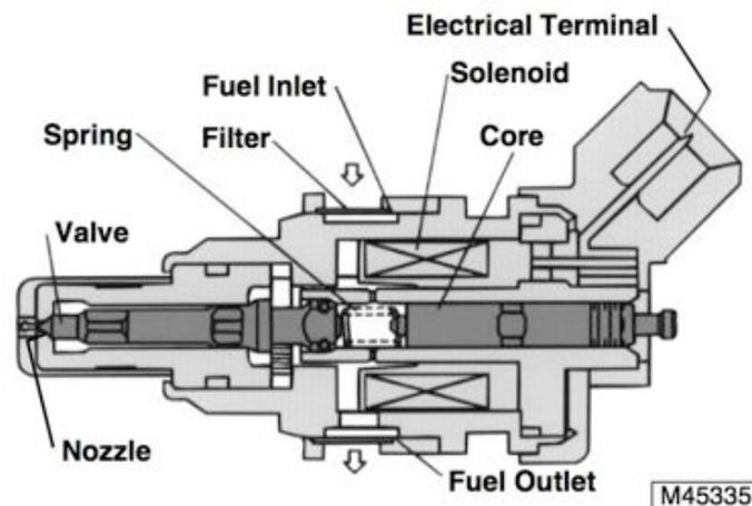
to be installed directly into the cylinder while others are designed to be installed in the intake manifold or the throttle body. It is important to also consider the injectors fuel flow capacity. An engine can be starved of fuel if the injector is too small, thus causing a power output decrease.
