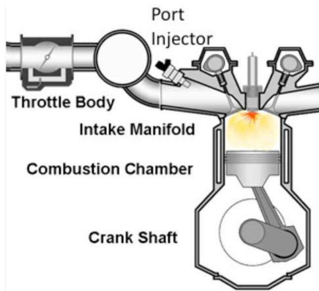
fuel is usually injected during the intake stroke while the intake valve is open. An oxygen sensor also communicates with the ECU to give closed loop feedback and make adjustments to regulate the air/fuel ratio (1).
