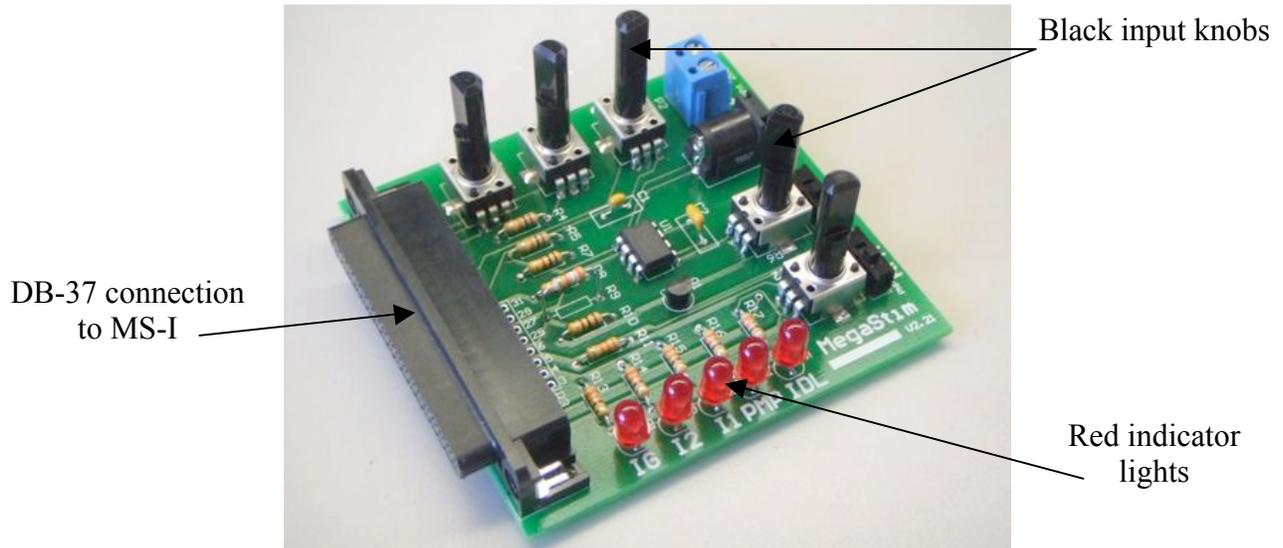
width, air/fuel ratio and duty cycle. There are five indicator LEDs on the bottom side. From left to right, they signal ignition, injector 2, injector 1, fuel pump and idle valve. When any of those are “on” then the respective LED will light up to signal the user.
