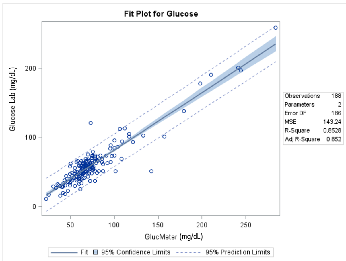
Figure 3. Fit plot illustrating 95% confidence and prediction limits for the whole blood glucose concentration from the CentriVet hand-held meter and the laboratory serum concentration
