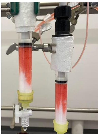
Figure 9 Columns showing channeling
