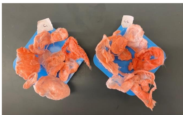
Figure 8 Cotton pulled apart showing uneven coating inside
